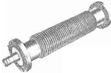
FLEXIBLE SECTION. ANDREW 19209B. Accommodates vibration and angles up to 30 degrees. Maximum offset is \frac{1}{2} ". Length, 18". Part No. 099 0441 000
